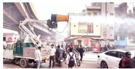
Anti-smog gun is used to spray water droplets to curb air pollution
